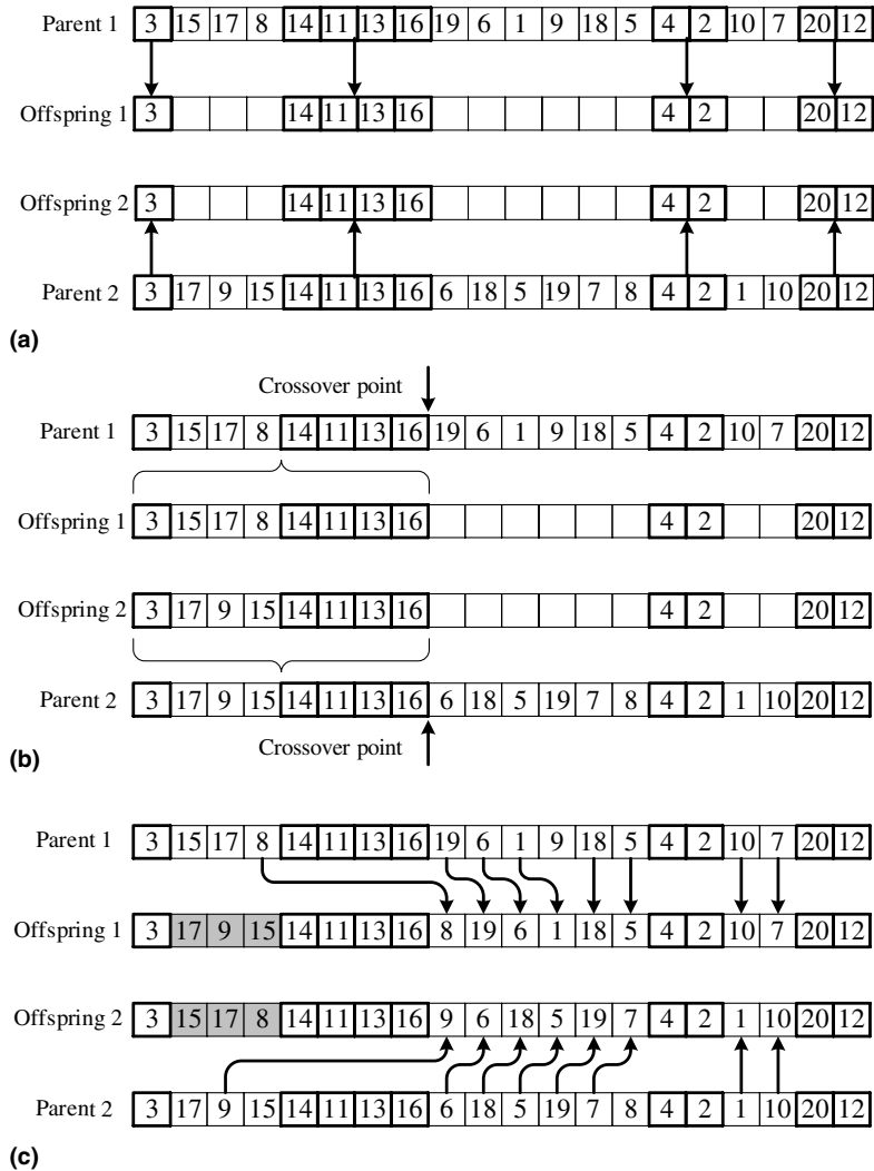
Fig. 1. “Similar Job Order Crossover” (SJOX): (a) first, the common jobs in both parents are copied over to the offspring; (b) then, jobs before a randomly chosen cut point are inherited from the direct parent; (c) the missing elements in the offspring are copied in the relative order of the other parent.
